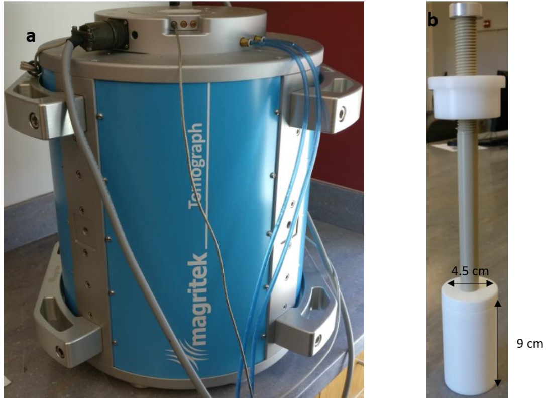
Figure 10: a) Table top low field MRI system used in this study. b) Sample holder and maximum sample dimensions.
