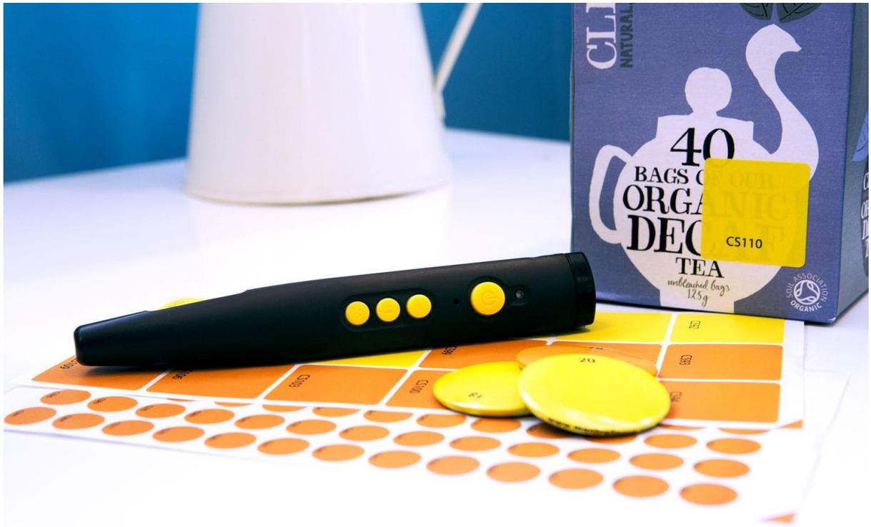
Figure 3: PenFriend with reusable magnetic braille labels
