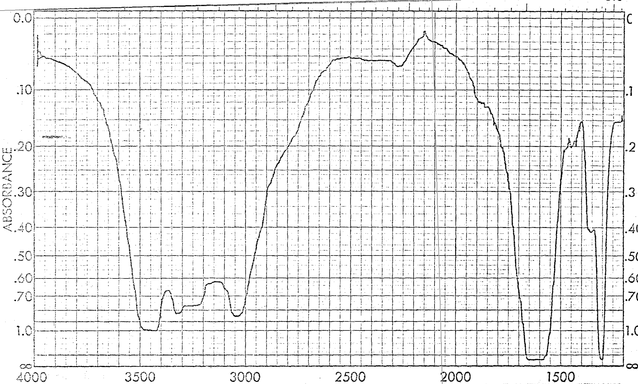
Spectrum No. 19: 50% Magnesium Ammonium Phosphate, MgNH_4PO_4 , and 50% Calcium Oxalate Monohydrate, CaC_2O_4 \cdot H_2O By Transmission I.R.
