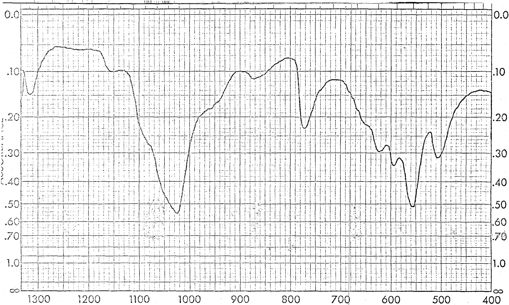
Spectrum No. 101: 25% Tricalcium Phosphate, \text{Ca}_3(\text{PO}_4)_2 , 25% Magnesium Ammonium Phosphate, \text{MgNH}_4\text{PO}_4 , 25% Calcium Oxalate Monohydrate, \text{CaC}_2\text{O}_4 \cdot \text{H}_2\text{O} , and 25% Magnesium Phosphate, \text{MgHPO}_4 by A.T.R.
