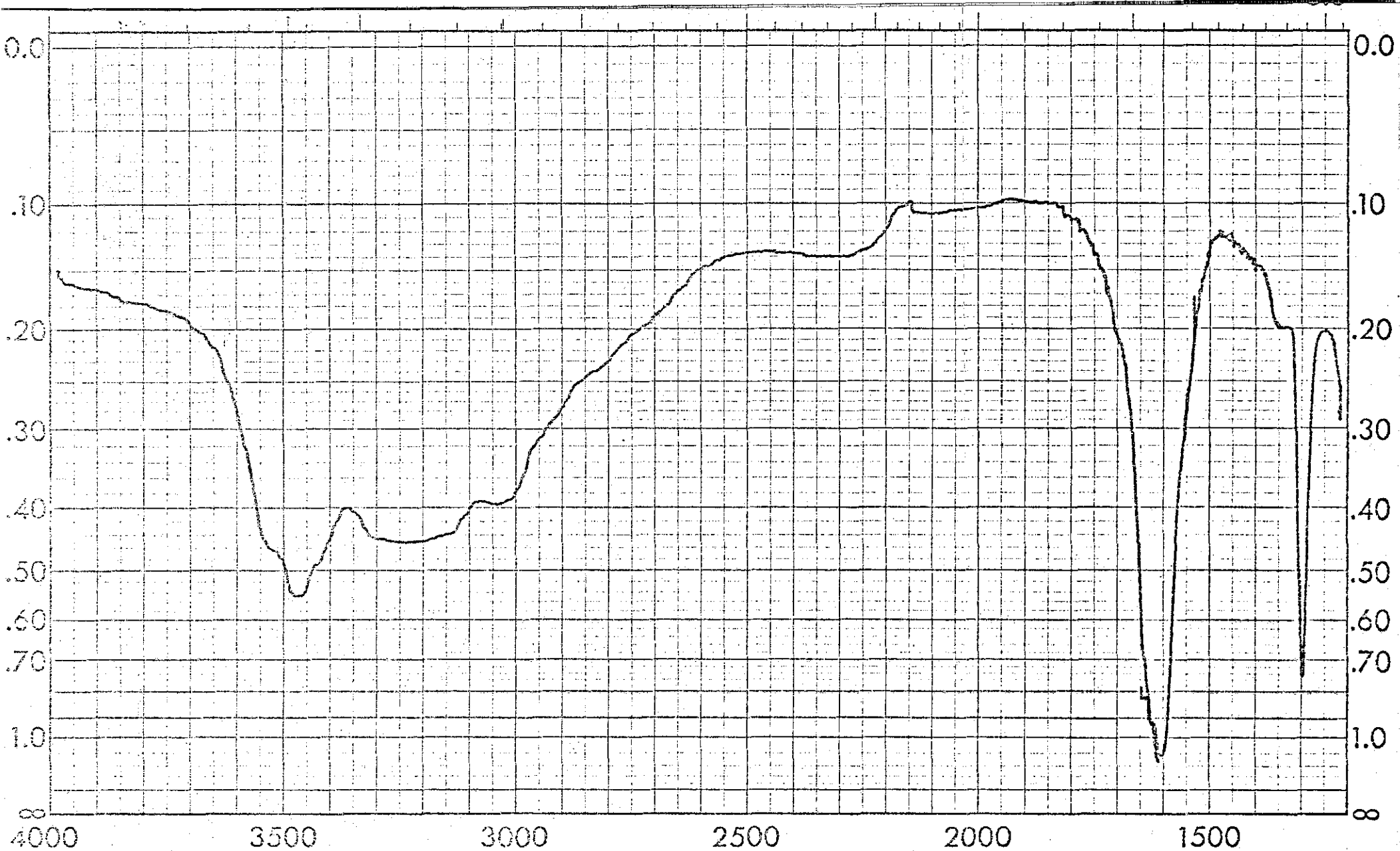
Spectrum No. 46: 50% Calcium Hydrogen Phosphate, \text{CaHPO}_4 , 25% Magnesium Ammonium Phosphate, \text{MgNH}_4\text{PO}_4 , and 25% Calcium Oxalate Monohydrate, \text{CaC}_2\text{O}_4 \cdot \text{H}_2\text{O} By Transmission I.R.
