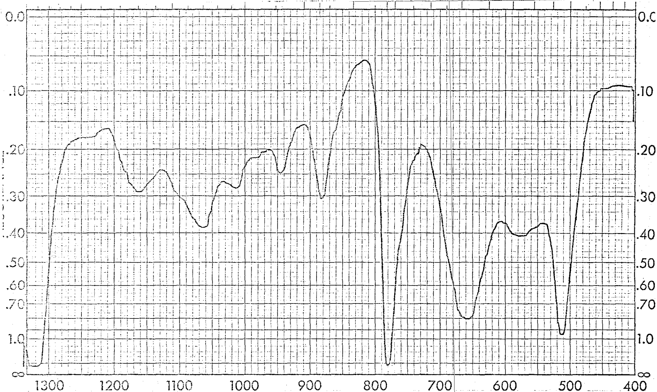
Spectrum No. 19: 50% Magnesium Ammonium Phosphate, \text{MgNH}_4\text{PO}_4 , and 50% Calcium Oxalate Monohydrate, \text{CaC}_2\text{O}_4 \cdot \text{H}_2\text{O} By Transmission I.R.
