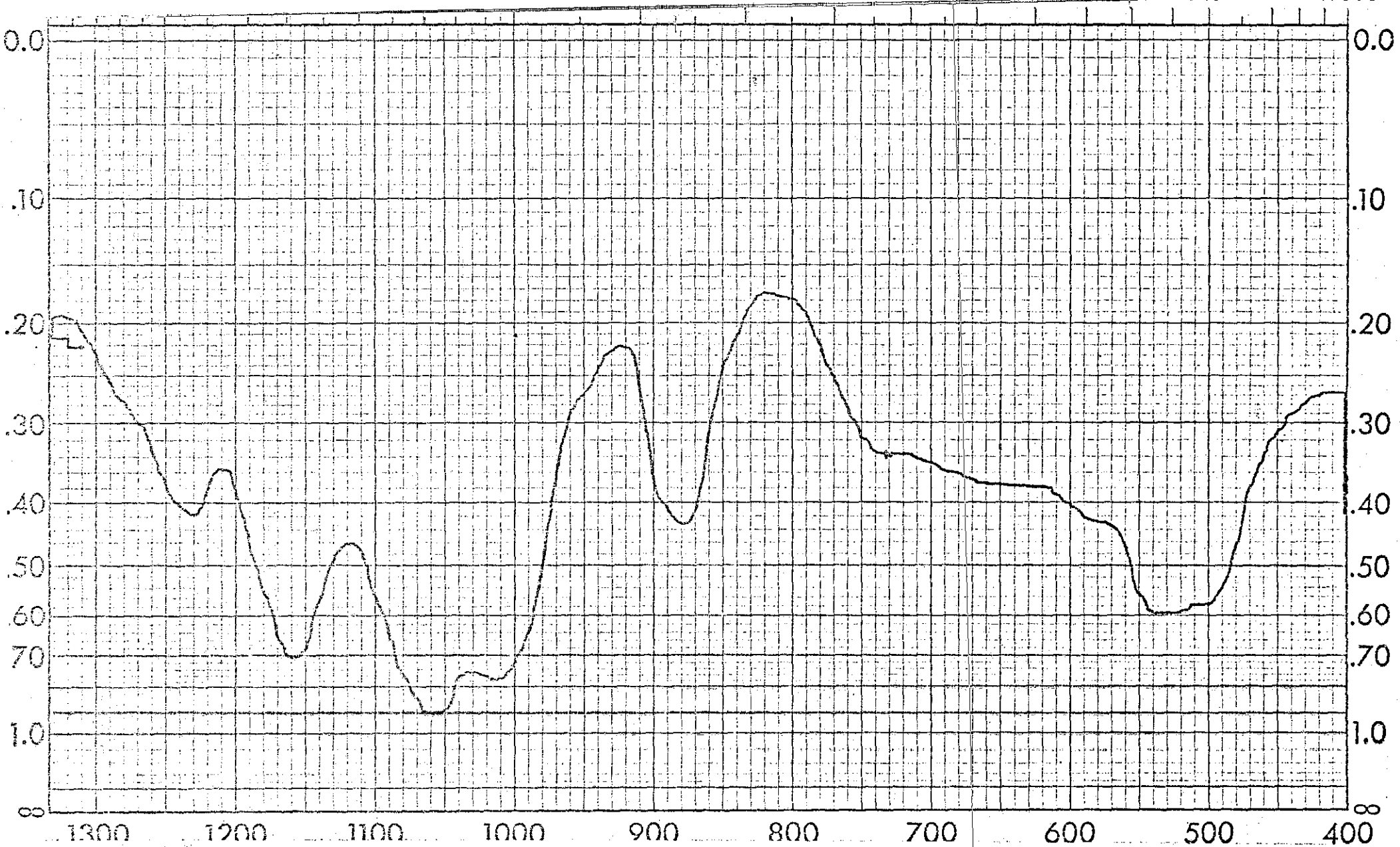
Spectrum No. 18: 50% Magnesium Ammonium Phosphate, \text{MgNH}_4\text{PO}_4 , and 50% Magnesium Phosphate, \text{MgHPO}_4 By Transmission I.R.
