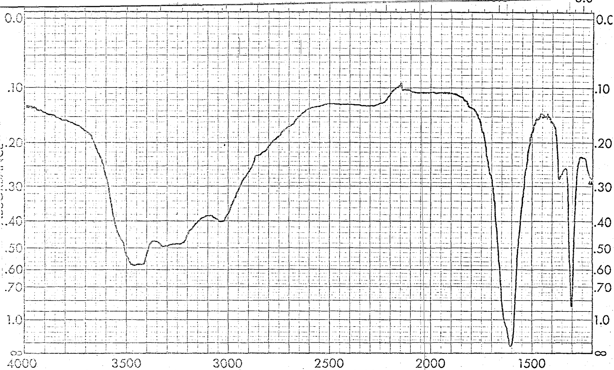
Spectrum No. 48: 25% Calcium Oxalate Monohydrate, \text{CaC}_2\text{O}_4 \cdot \text{H}_2\text{O} , 25% Calcium Hydrogen Phosphate, \text{CaHPO}_4 , 25% Tricalcium Phosphate, \text{Ca}_3(\text{PO}_4)_2 , and 25% Magnesium Phosphate, \text{MgHPO}_4 By Transmission I.R.
