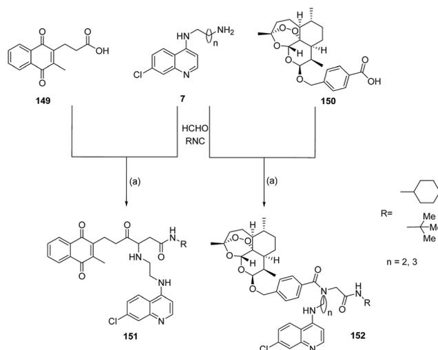
Scheme 23 Reagents and conditions: (a) succinic acid, silver nitrate, ammonium persulfate, 30% aq. CH<sub>3</sub>NH<sub>2</sub>, 65–70 °C, 3 h.
