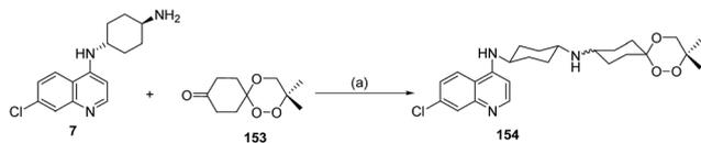
Scheme 24 Reagents and conditions: (a)  $\text{NaBH}_3\text{CN}$ , MeOH, HCl/i-PrOH.
