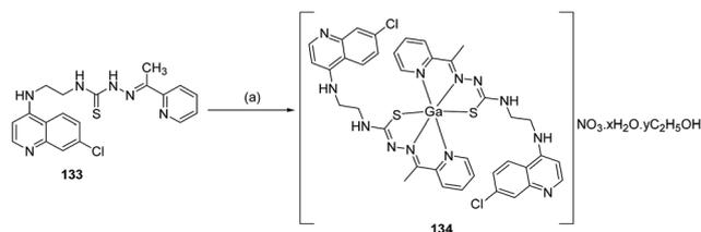
Scheme 18 Reagents and conditions: (a)  $\text{Ga}(\text{NO}_3)_3 \cdot \text{H}_2\text{O}$ , ethanol, reflux, 2 h.
