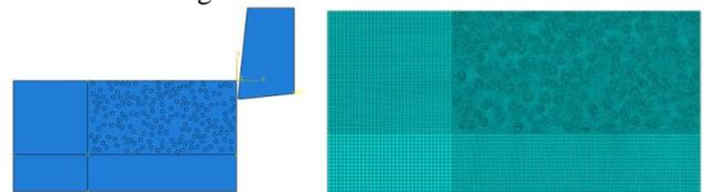
(a) Multi particle cutting assembly (b) grid generation
