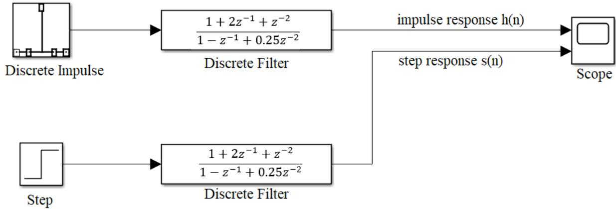
Figure 1: OER lab exploring impulse response and step response of systems
