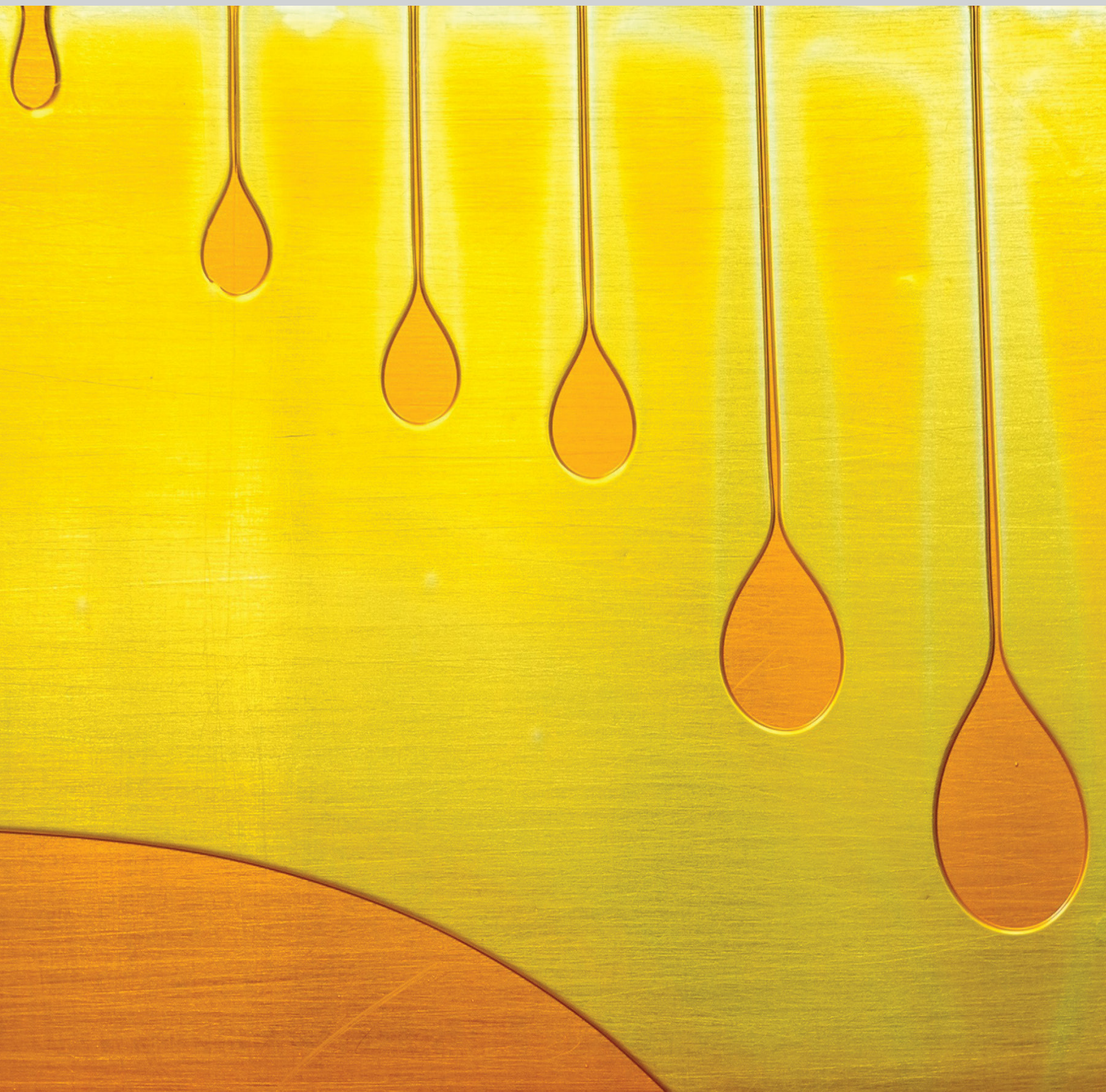
Dyed glycerin parcels between parallel glass plates separate from the top edge and flow as droplets, demonstrating fluid instability.
