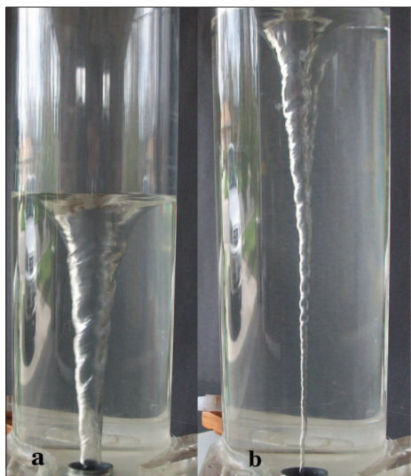
Fig. 2. Bathtub vortex with (a) fully open outlet and (b) partially open outlet.
