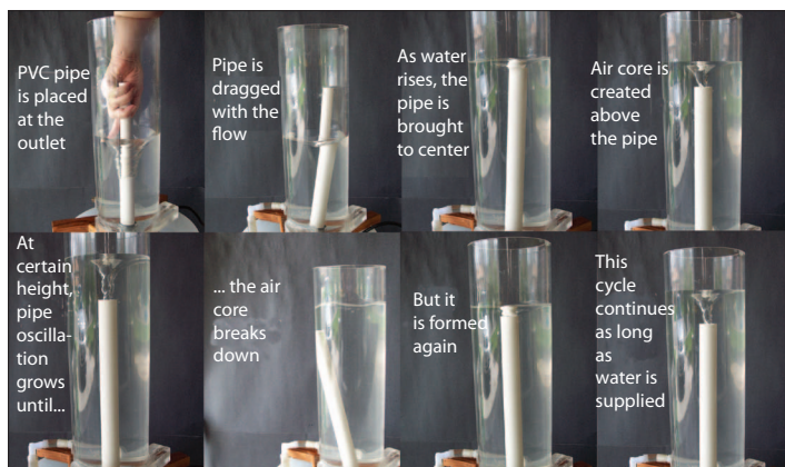
Fig. 5. The sequence of self-induced vibration of a pipe in BTV. Photos to be viewed from left to right, top row first.
