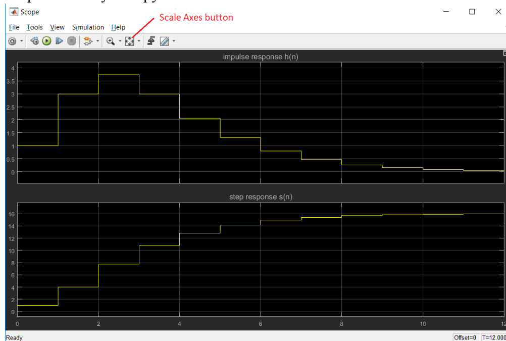
Fig. 5. Impulse response and step response of the discrete filter
