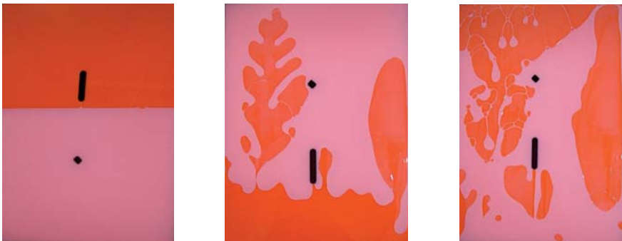
Figure 2 – From left to right, sequence of operation from idle and stable condition to ever-changing patterns. Large bubbles are formed after a very long idle (middle image)
